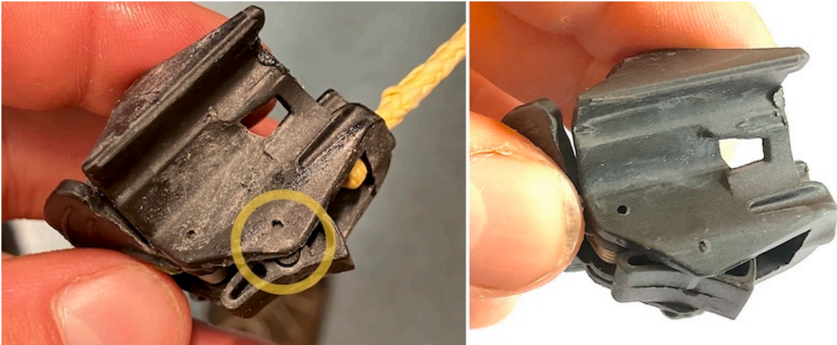
Figure 3.4: Sliders with broken axle on pawl (left) and intact axle on pawl (right)
