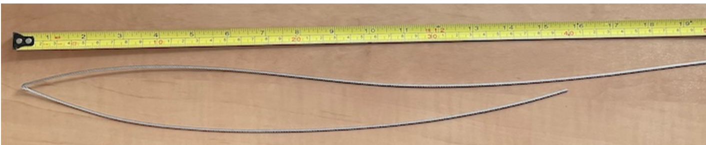
Figure 4.21: 1.5mm 7x7 stainless steel wire rope with sharp bend
