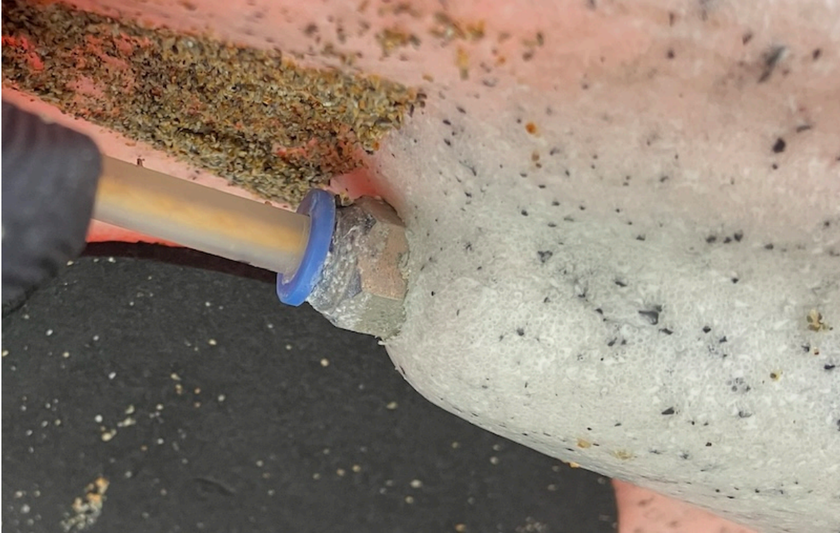
Figure 4.5: Pneumatic line fitting in plastic boat with skudder-type skeg
