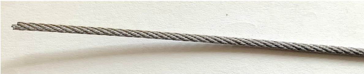
Figure 4.20: 1.5mm 7x7 stainless steel rope
