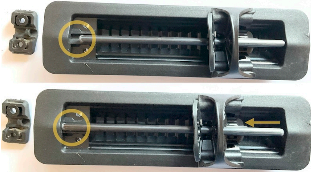
Figure 3.2: 2.Slide the bar forwards to release it from the hole at the back of the ratchet box. Remove the bar with the slider on it.
