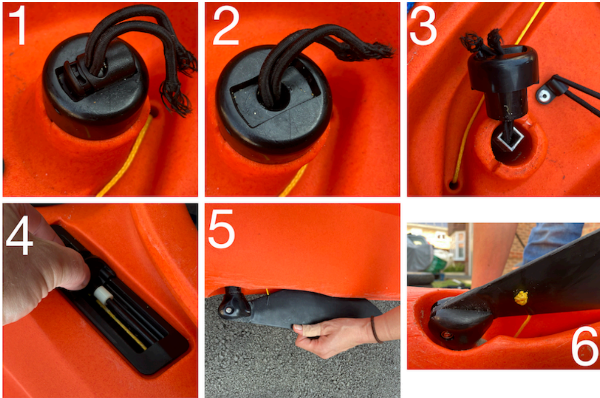
Figure 5.8: Removal of the skudder-type skeg blade assembly
