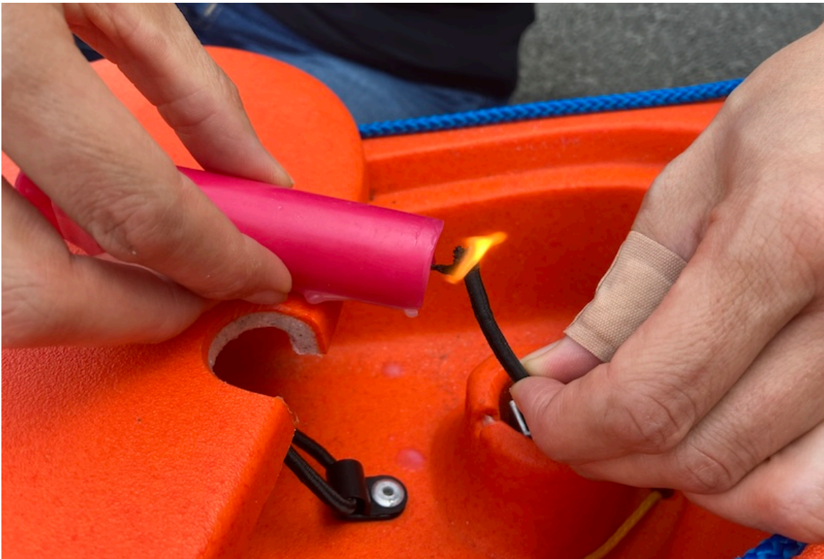
Figure 5.9: Sealing the blade elastic ends using a candle
