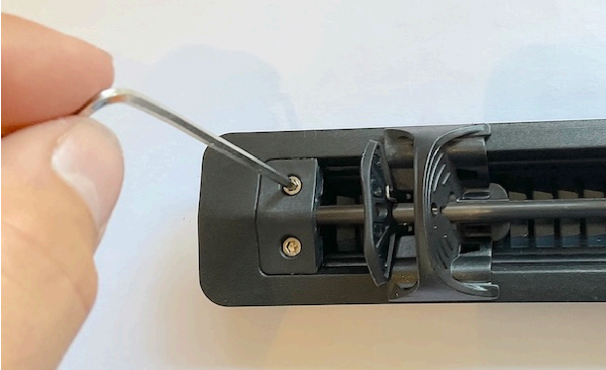
Figure 3.9: Tighten the screws. Do not over-tighten - max torque = 1.5 Nm (until you feel some resistance and then an another quarter turn, it should be sufficient to only hold the short end of the Allen key)
