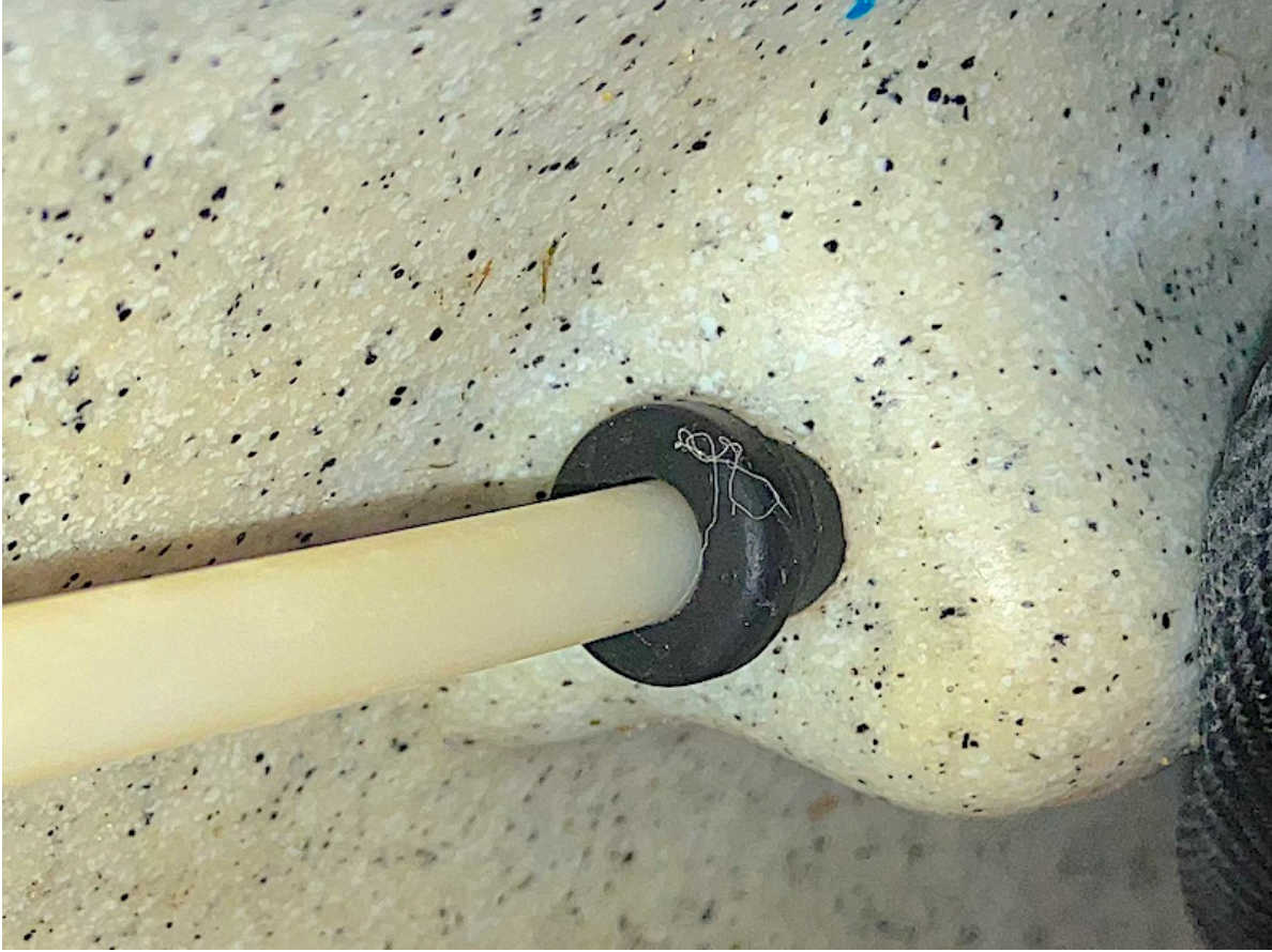
Figure 4.8: 8mm tube running to slider box with grommet
