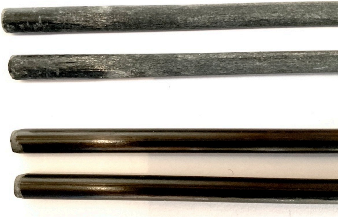
Figure 3.6: Two worn rods (top) and two new rods (bottom)
