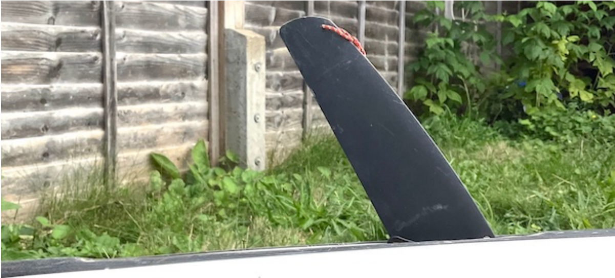
Figure 3.10: Deployed blade (slider fully back) at (approximately) correct adjustment - around 70° to the boat, with the lower cord hole in the blade just visible.
