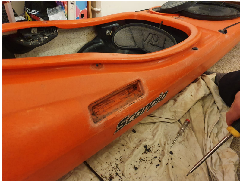
Figure 3.11: Controller recess in boat, with ratchet box removed and most of the adhesive residue scraped away.
