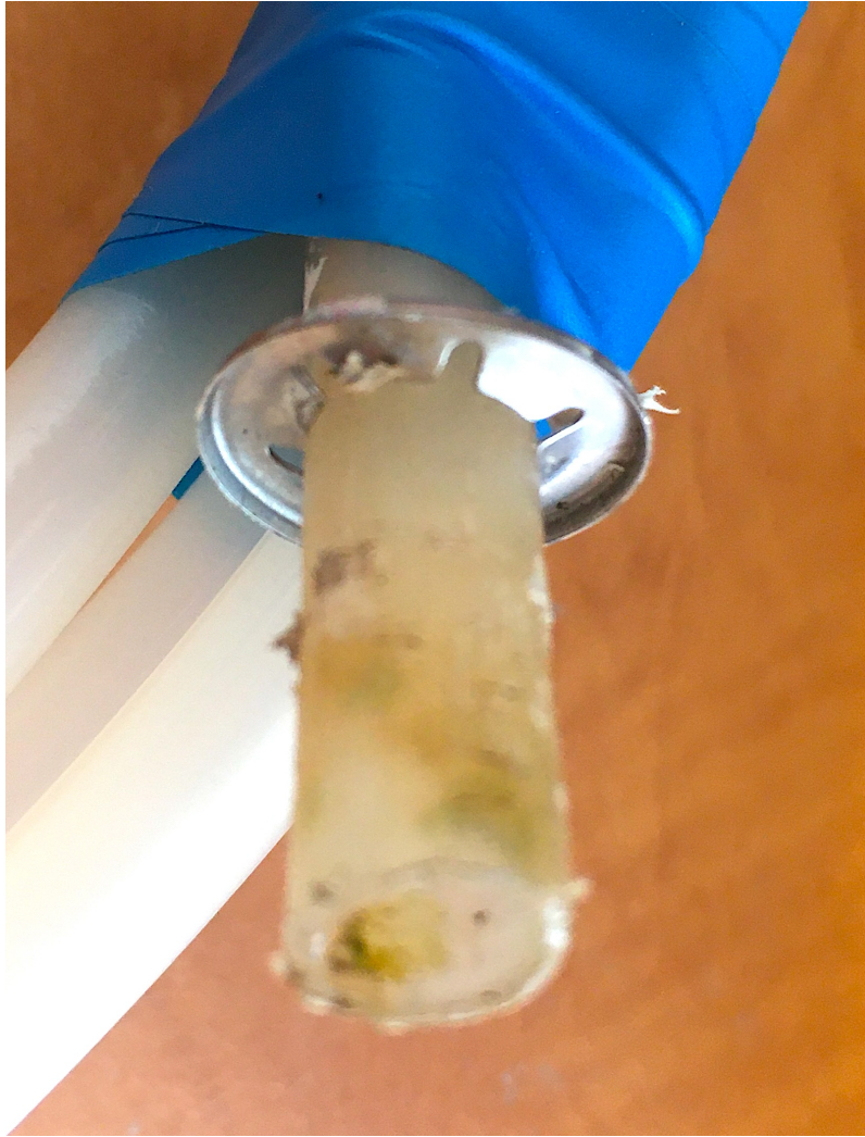
Figure 4.16: Star nut pressed on to tube end
