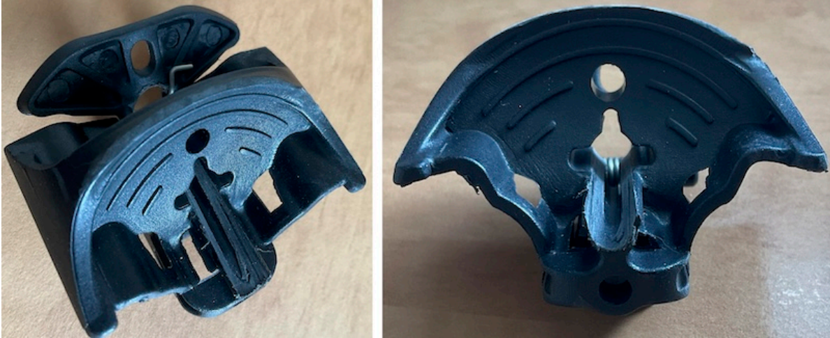
Figure 3.5: Button worn where it contacts the bar
