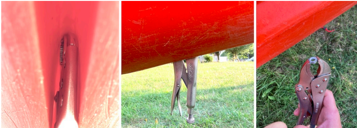
Figure 4.12: Using mole grips to grasp the nut on the compression fitting
